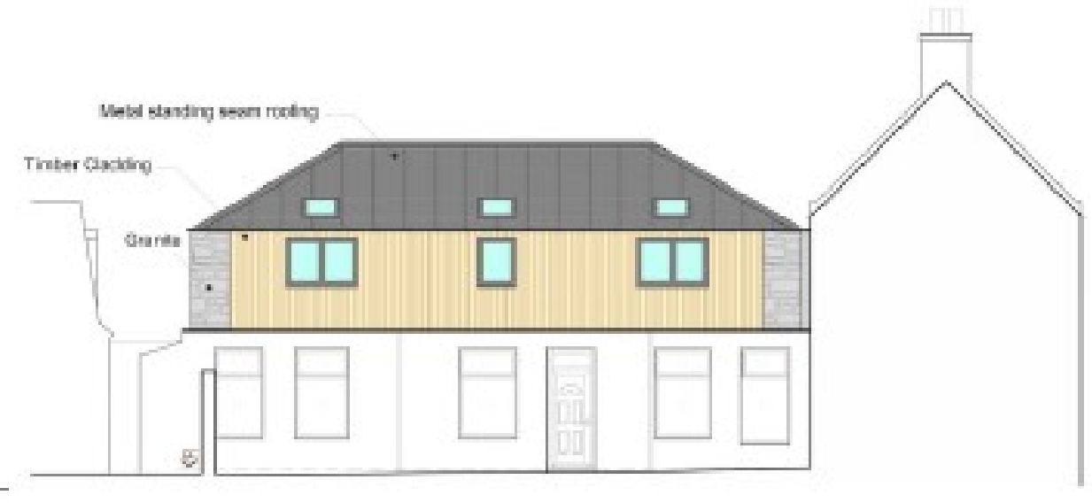
South West Elevation - 1:100
